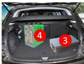
3. HHO generator and DC TO AC inverter is install in the luggage room of the car
