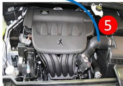
4. HHO gas pipe insert into the air inlet.
