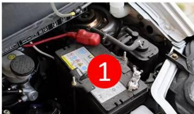
1. BATTERY of car is install in the engine room
