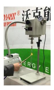
Automatic rotary sealing: oxyhydrogen generator with quartz tube sealing machine to complete the sealing, vacuuming, gas filling at a time.
