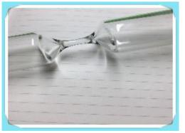
Step 1: Heat and soften the quartz glass, and pull it into a "8" shape.
