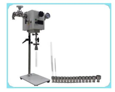
Quartz tube vacuum sealing device is used for vacuum sealing samples under oxygen-free and water-free conditions by dynamic sealing technology. Quartz tube is vacuumed during auto rotating and inert gas filling at the same time, which is easy to operate, with high vacuum and high sealing efficiency.
