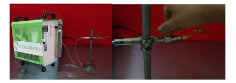
3. Adopt lighter to fire the oxy-hydrogen gas for flame, user can adjust the valve to control the flame.(Attention: when fire the gas, don't let any parts of your body in the front of the flame nozzle in case burnt ;when use lighter , user need fire from the side of the flame torch in case burnt your hand.
