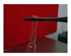
5. Put the bottle which clamped by the tweezers to the oxy-hydrogen gas flame for heating .Rotate the bottle while heating .When the bottle is heat ,pull up the bottle head by tweezers, then bottle is sealed. Please see the video by the link <a href="http://www.okayenergy.com/video/product-video/65.html">http://www.okayenergy.com/video/product-video/65.html</a>
